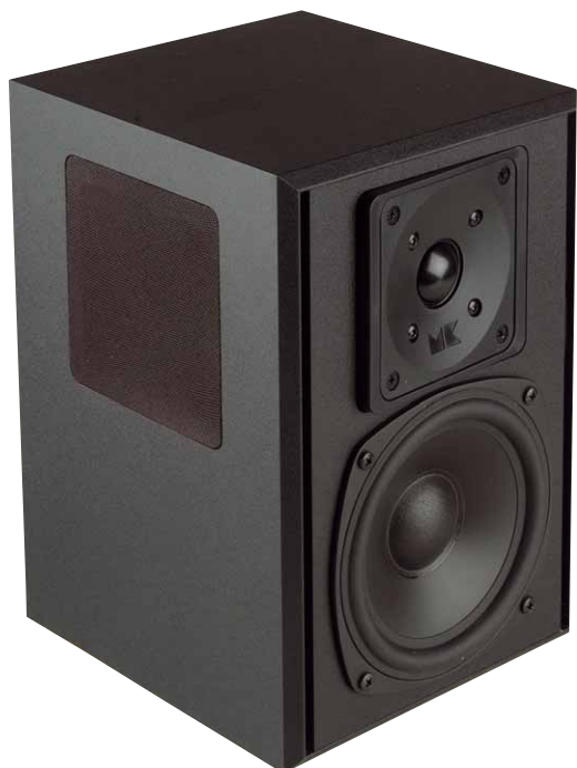
The rear speakers of the M&K set are real tripoles: In addition to a direct-beam 2-way system, two broadband drivers built into the side walls ensure the desired diffuse sound of the surround channels
