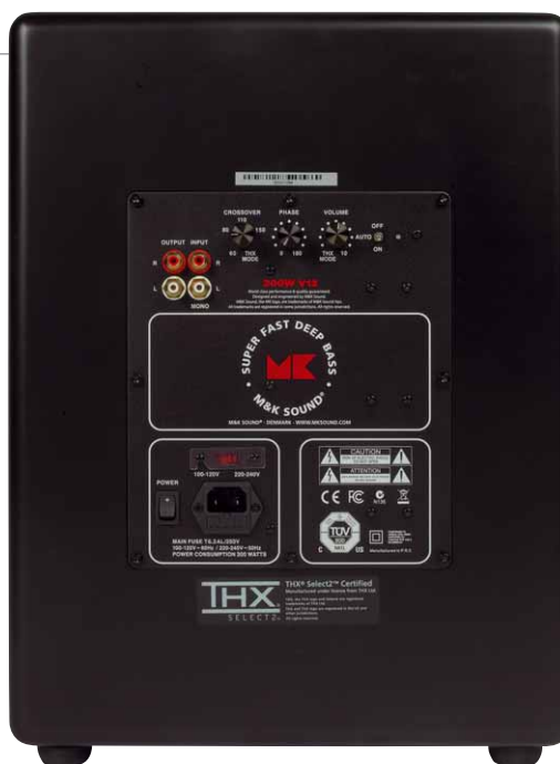
The approximately 300 watt amplifier module of the V12 subwoofer provides the standard settings for level, phase and crossover frequency. Unfortunately, the V12 does not have a remote control or EQ setting on board
