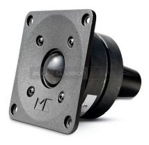
At first glimpse, the tweeter appears to be a standard 1" dome, but beneath the surface it conceals technical solutions required to deliver high performance, such as the large, damped air chamber behind the dome. The ability to withstand higher output is also attested by the vents of the voice coil and the copper-coated aluminium coil, which is lighter than copper wires.
