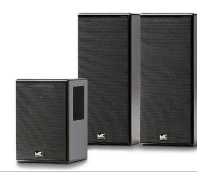
older speaker is cube-shaped and has an angled front baffle, the LCR950 is rectangular (16 inches high by 7 inches wide) with a straight-on front baffle. In keeping with MK's design philosophy of keeping the front baffle as small as it can be in order to manipulate baffle-related diffraction that can affect the sound of the speaker, the LCR950 is just a bit wider than the midbass drivers themselves. The tweeter is a new one developed for a couple of MK's pro monitors,
