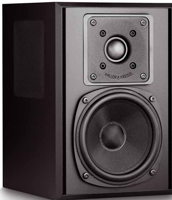
The rear speakers of the M&K set are true tripoles: In addition to a direct-radiating 2-way system, two full-range drivers built into the side walls provide the desired diffuse sound for the surround channels.
