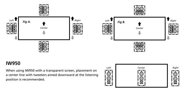
When using IW950 with a non-transparent screen, the center channel can be placed horizontally above or below the screen, while the Left and Right speakers may be moved up or down to approach the horizontally placed center channel position.
