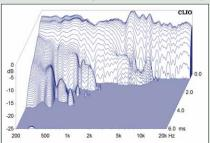
Like virtually no other speakers, the M&K Sound S300 distinguish themselves through an almost berfect waterfall diagram. Even at low frequencies they produce virtually no post oscillation.
